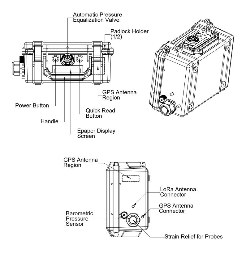
Duro UAS Field Sonde V2.1 Weight: 5.7 lbs Dimensions: 8.7 in x 6.2 in x 3.9 in (LxWxH) Model courtesy of Shane Davis at GrabCAD
