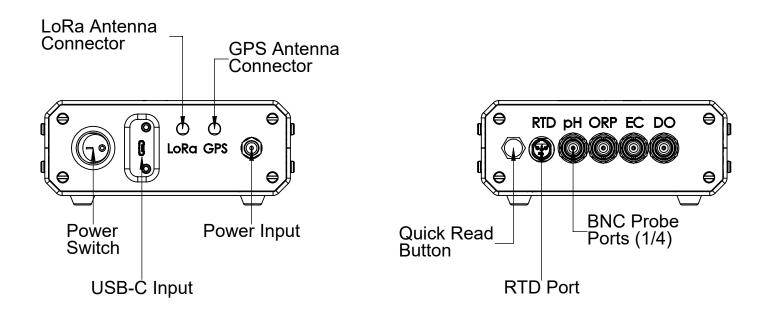
Duro UAS Lab Sonde V2.1 Weight: 2.1 lbs Dimensions: 7.1 in x 5.3 in x 2.2 in (LxWxH)
