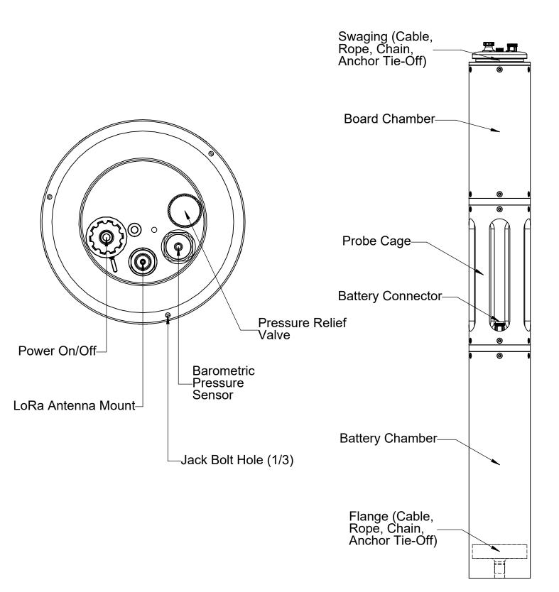
Duro UAS Nearshore Sonde V2.1 Weight: 13.7 lbs (w/o batteries) | 20.2 lbs (w/ batteries) Dimensions: Length = 38.5 in | Diameter = 4.5 in
